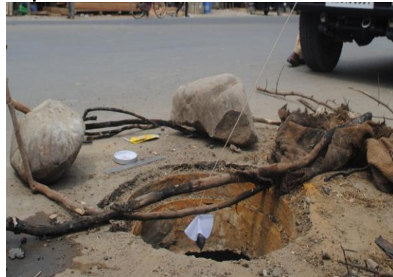
Fig. 5: Lead Acetate Paper Test for Hydrogen Sulphide
