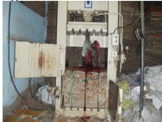
Fig. 6: Scene of Accident Showing the Body trapped in Situ in Baler Machine
